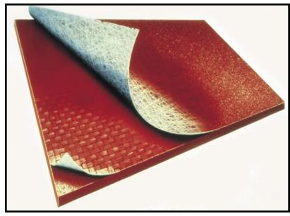
Fibergrate and Chemplate are manufactured by building up multiple layers of fiberglass reinforcement and specially-formulated resins. The result of this process is a solid composite panel offering both bi-directional strength and corrosion resistance.
