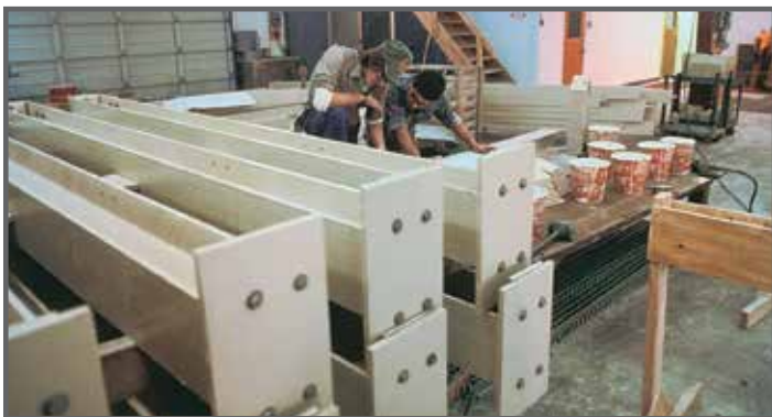
Fabricated Dynaform columns ready for shipment.
