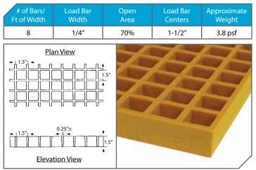
Section Properties per Ft of Width: A = 2.85 IN<sup>2</sup> I = 0.51 IN<sup>4</sup> S = 0.65 IN<sup>3</sup>
