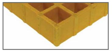
Meniscus Top: The concave surface of Fibergrate<sup>®</sup> meniscus top grating provides superior slip resistant footing in most environments including wet or oily conditions. It is the standard surface for most Fibergrate molded gratings.
