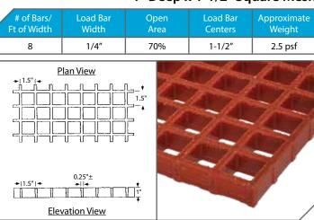
Section Properties per Ft of Width: A = 1.71 IN<sup>2</sup> I = 0.14 IN<sup>4</sup> S= 0.29 IN<sup>3</sup>
