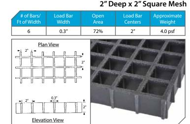
Section Properties per Ft of Width:  $A = 2.88 \text{ IN}^2$  I = 0.96 IN<sup>4</sup> S = 0.94 IN<sup>3</sup>
