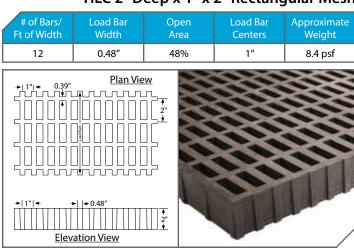
Section Properties per Ft of Width:  $A = 10.26 \text{ IN}^2$   $I = 3.4 \text{ IN}^4$   $S = 3.27 \text{ IN}^3$
