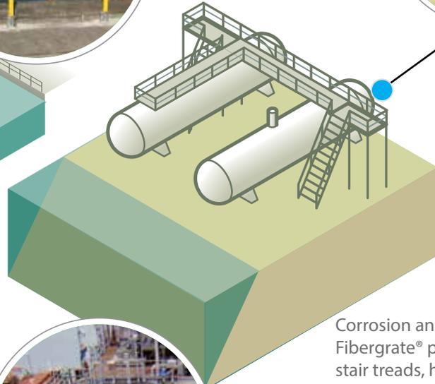
Corrosion and slip resistant Fibergrate® products including stair treads, handrail, grating, and structural profiles provide access platforms to processing tanks located on the shoreline.
