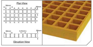
Section Properties per m of Width:  $A = 6.03x103mm^2$   $I = 6.96x10^5mm^4$   $S = 3.49x10^4mm^3$
