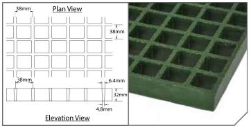
Section Properties per m of Width: A = 4.57x103mm<sup>2</sup> I = 4.37x105mm<sup>4</sup> S= 2.58x104mm<sup>3</sup> \*Not available with meniscus top surface (only grit)
