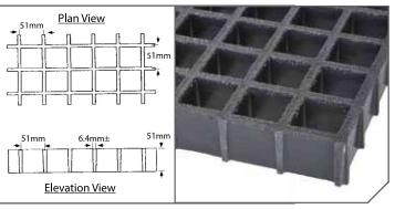
Section Properties per m of Width:  $A = 6.10 \times 103 \text{mm}^2$   $I = 1.31 \times 10^6 \text{ mm}^4$   $S = 5.05 \times 10^5 \text{mm}^3$
