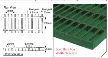
Section Properties per m of Width: A = 5.44x103mm<sup>2</sup> I = 3.00x10<sup>5</sup>mm<sup>4</sup> S= 2.31x10<sup>4</sup>mm<sup>3</sup>
