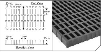
Section Properties per m of Width:  $A = 1.58 \times 10^4 \text{mm}^2$   $I = 1.90 \times 10^6 \text{mm}^4$   $S = 9.68 \times 10^4 \text{mm}^3$
