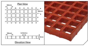
Section Properties per m of Width: A = 3.62x103mm<sup>2</sup> I=1.91x10<sup>5</sup>mm<sup>4</sup> S=1.56x10<sup>4</sup>mm<sup>3</sup>
