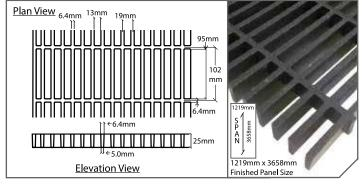
Section Properties per m of Width: A = 7.58x103mm<sup>2</sup> I = 4.07x10<sup>5</sup>mm<sup>4</sup> S= 308x10<sup>4</sup>mm<sup>3</sup>
