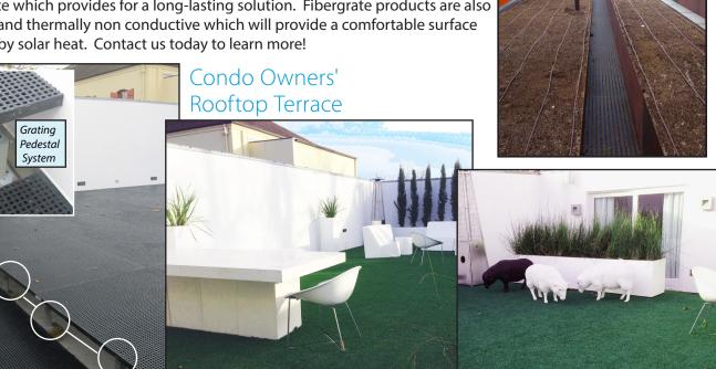
Micro-Mesh® grating and pedestals create a level, elevated rooftop terrace that ensures corrosion resistance and proper drainage. The grating surface was covered by artificial turf and outdoor furnishings increasing the owners' living space while providing low maintenance landscaping.
