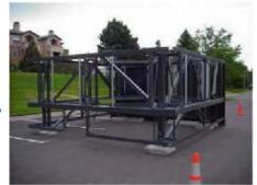
(4' antenna separation per sector, 13° mechanical down-tilt)
