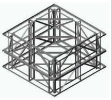
Completed Screen (Shown as 8' tall unit) - structural framing for antenna mounting and RF plate supports, cross-bracing and RF fiberglass cladding. All materials are fiberglass - lightweight and RF transparent, including access door.
