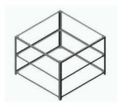
Basic Leg Frame - note (4) legs in corners. By simply changing these four elements, the basic upper 5' structure can be modified from 5' to 10' in 1' increments. Leg extension kits are available for all standard designs.
