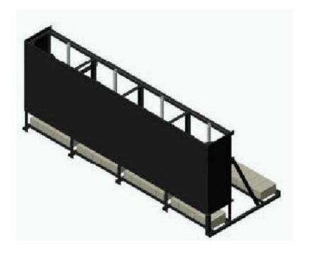
**Completed Single-Sector Screen** - structural framing for antenna mounting and RF plate supports, cross-bracing and RF fiberglass cladding. All materials are fiberglass - lightweight and RF transparent.
