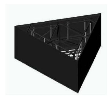
**Completed Triangle RF Screen** - structural framing for antenna mounting and RF plate supports, cross-bracing and RF fiberglass cladding. All materials are fiberglass - lightweight and RF transparent.
