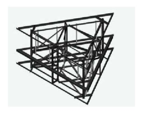
Triangle Structure (including additional framing and cross-bracing) - note (3) legs in corners. By simply changing these three elements, the basic upper 5' structure can be modified from 5' to 10' in 1' increments. Leg extension kits are available for all standard designs. Note antenna mounting hardware pipes (2.5" galvanized steel) are included.
