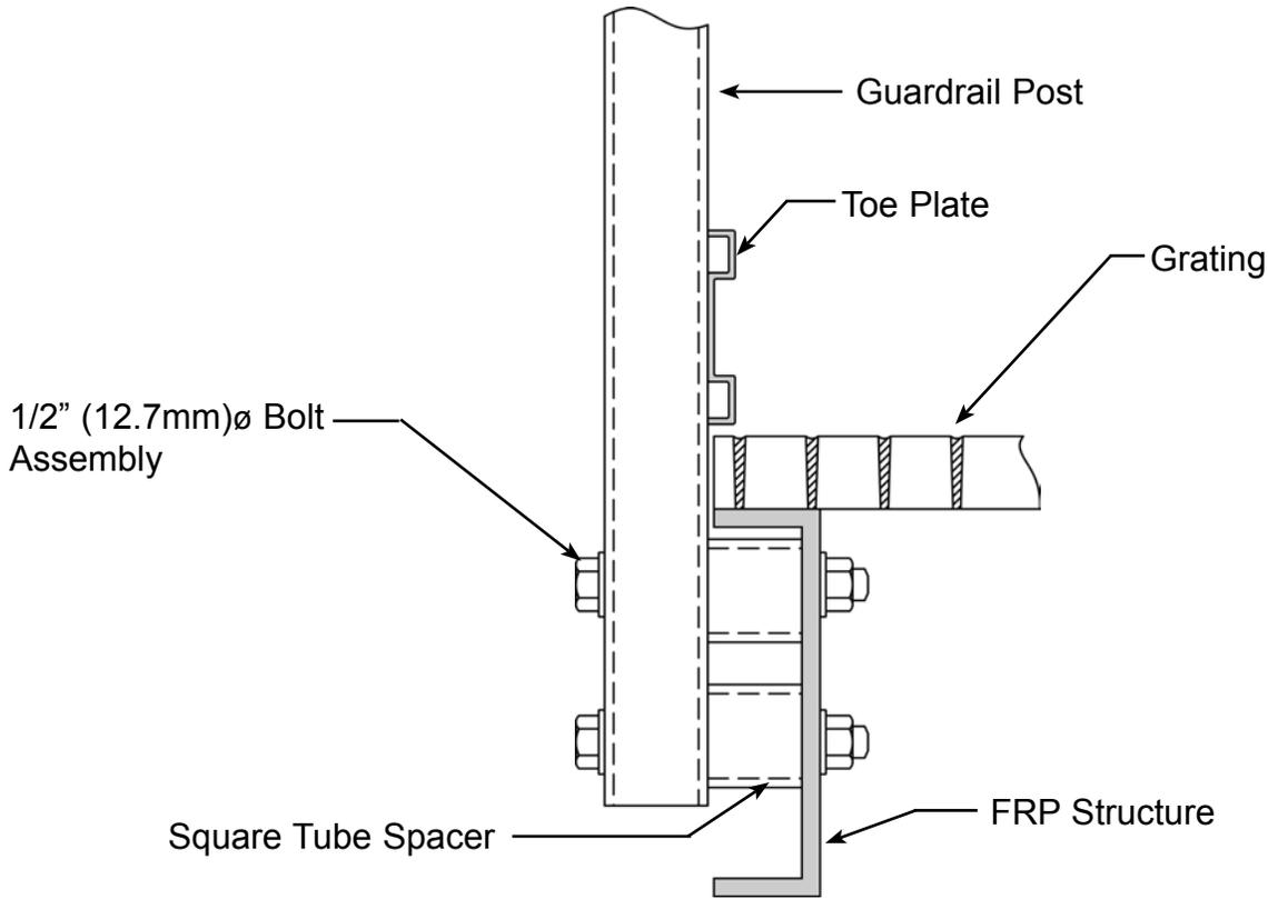
**DRAWING L: REMOVEABLE GUARDRAIL CONNECTION**
